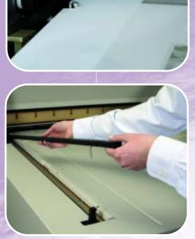
The MAKO 8 is designed to facilitate maximum format flexibility. The MAKO 8 can accommodate any plate size between 32.4" x 45.0" (824mm x 1143mm) and 10.0" x 10.0" (254 mm x 254 mm). The largest format provides generous space for 8-page jobs with all trim marks and color bars in position. The minimum format allows for most popular duplicator size presses.
